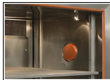
C-rails, shelves, lighting
